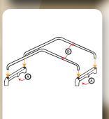
STEP 5 Gently push 2 x arches D Into the top of 2 x cross sections A, as shown in the image, forming an arch frame.
