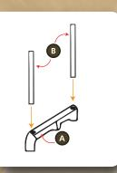
STEP 1 Gently push 2 x B into the top of cross section A.
