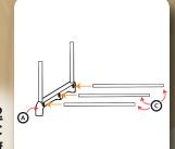
STEP 2 Gently push 3 x C into the side of cross section A.
